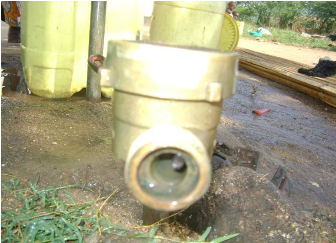
Figure 5: Part of a stick inserted in a water meter to prevent it from measuring consumed water
