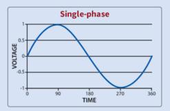
With the wave form of single-phase power, when the wave passes through zero, the power supplied at that moment is zero. The wave cycles 50-60 times per second depending on your location.
