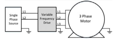
Figure 4. Schematic of Variable Frequency Drive
