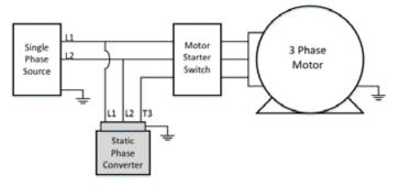
Figure 1. Schematic of 3-phase static converter installation
