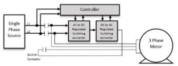
Figure 3. Schematic of digital 3-phase converter
