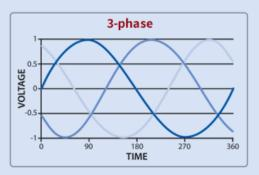
3-phase power has 3 distinct wave cycles that overlap. Each phase reaches its peak 120 degrees apart from the others so the level of power supplied remains consistent.
